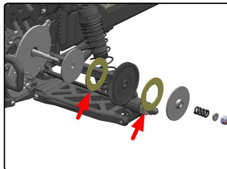
Replace the slipper pad #C-00250-088
