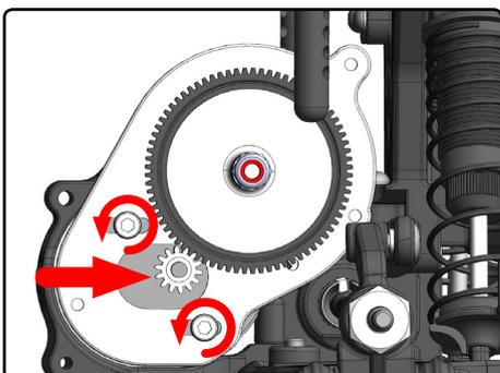
Loosen the motor screws.
